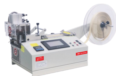
V-120LRQ Pneumatic belt loop cutter cold & hot knife
