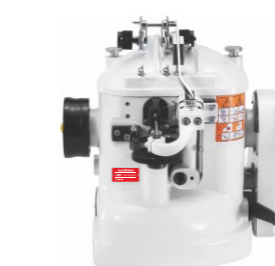
V-GP800-2 Heavy duty lubrication over-seaming machine single needle double thread widely use, such as diving suits, leather, fur, sheep skin and double face combination of fur and fabric, edging collars, sleeves and foreparts, with 2 thread chain stitch.
