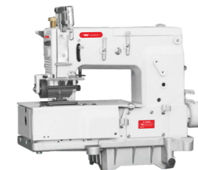
V-1423P 1/8 twenty three needles with vertical looper movement 3/16 needle gauge distance reach 108.8mm between first and last needle 1/4 needle gauge distance reach 152mm between first and last needle
