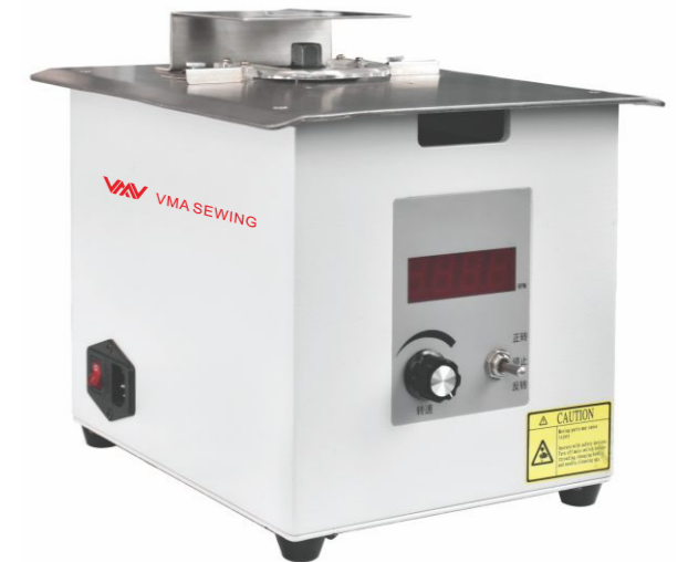
V-PF130A Double face cashmere splitting machine, automatic adjust knife, 130mm size knife, servo motor, cutting width 1.1-15mm, 2000-11000rpm, 550W 220V.
