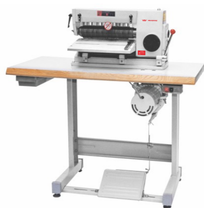
V-512-2 Cutting leather strip cutting width 16" inch 400mm, speed 10m/min, adjustable strip width, knife 80x40x1mm, 380/220V, 135/150kg. Also cutting width have 14 inch 345mm and 20 inch 508mm.
